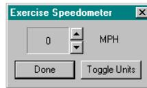
While the tool is in the exercise gauge mode, it will continuously broadcast ATA data link messages to simulate an engine or a vehicle operating condition. However this mode is only useful if the instrument panel cluster that is under service has been programmed to operate from the ATA data link. No other tool feature is made available until the exercise gauge mode is complete by clicking on the **Done** button.
